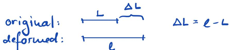
engineering strain:  $e = \frac{\Delta L}{L} = \frac{l - L}{L}$
