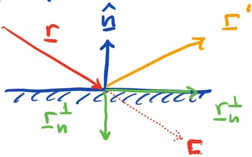
$$\begin{aligned} \underline{\underline{r}}' &= \underline{\underline{r}}^{\perp} - \underline{\underline{r}}^{\parallel} \\ &= \underbrace{(\underline{\underline{I}} - 2 \underline{\underline{\hat{n}}} \otimes \underline{\underline{\hat{n}}})}_{\underline{\underline{M}}_n} \underline{\underline{r}} \end{aligned}$$
