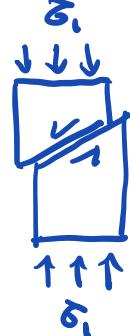
Empirical criterion that allows prediction of shear failure.
