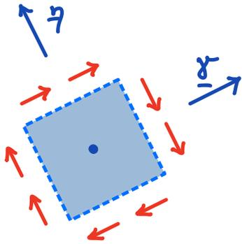
$$\underline{n} = \underline{\eta}: \underline{\underline{\sigma}} \underline{n} = \tau \underline{\gamma}$$
