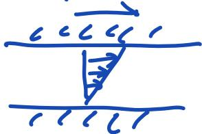
$$\underline{\underline{\sigma}} = \begin{bmatrix} 0 & \sigma_s & 0 \\ \sigma_s & 0 & 0 \\ 0 & 0 & 0 \end{bmatrix}$$
