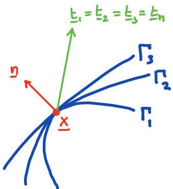
This assumes that the traction field is independent of  $\nabla \underline{n}$  and hence the curvature of the surface. Therefore the traction  $\underline{t}_i$  on the set of surfaces  $\Gamma_i$  that are tangent at  $\underline{x}$  is the same,  $\underline{t}_i = \underline{t}_n$ .
