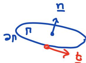
$$\int_{\Gamma} (\nabla \times \underline{v}) \cdot \underline{n} dA = \oint_{\partial\Gamma} \underline{v} \cdot \underline{t} ds$$
