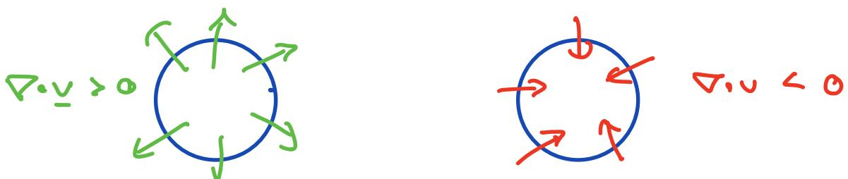
Incompressible flows & deformations are solenoidal  $\nabla \cdot \underline{v} = 0$
