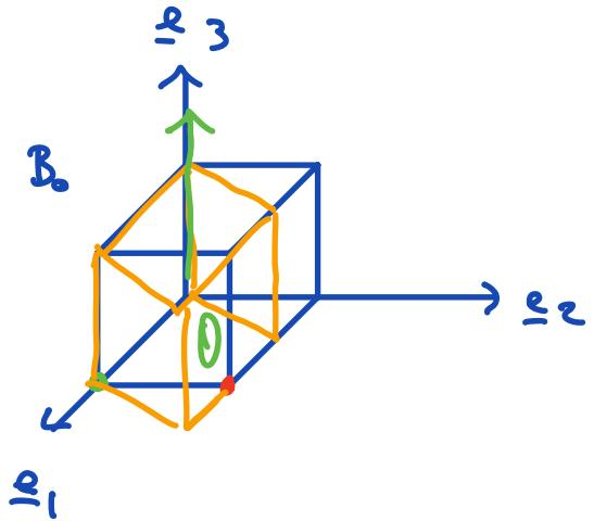
$$\underline{x} = \underline{\varphi}(\underline{x}) = \begin{bmatrix} x_1 + \alpha x_3 \\ x_2 \\ x_3 \end{bmatrix} =$$
