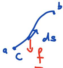
$$W = \int_{t_1}^{t_2} f \cdot \underline{v} dt = \int \frac{dW}{dt} dt \Rightarrow \frac{dW}{dt} = f \cdot \underline{v}$$
