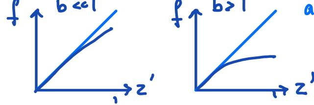
$$f(z) = -\frac{E_a}{RT_B} \frac{1}{1 + \frac{\Delta T}{T_B} \frac{z}{H}} \approx -\frac{E_a}{RT_B} \left(1 - \frac{\Delta T}{T_B} \frac{z}{H}\right)$$
