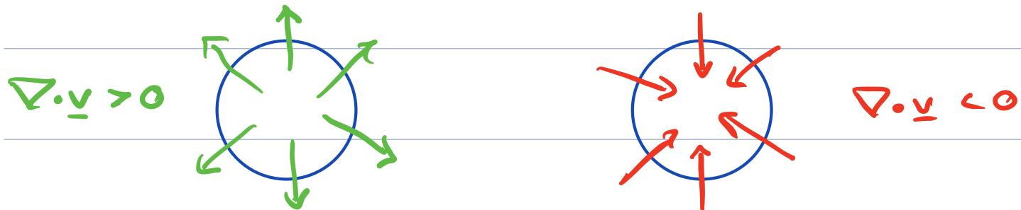
Incompressible flows/deformations are solenoidal  $\nabla \cdot \mathbf{v} = 0$ .
