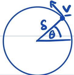
$$\text{angular velocity: } \omega = \frac{d\theta}{dt}$$
