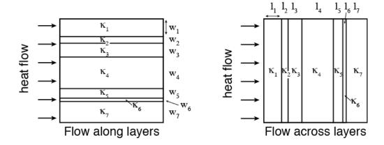
Consider a material with *N*layers, where the n-th layer has thermal conductivity,  $\kappa_n$ , and width or length,  $w_n$  or  $l_n$ , depending on flow direction. The total width or length of the material are therefore
