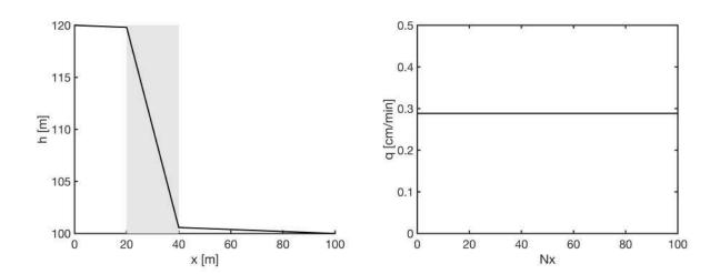
The solution shows that most of the head drop occurs in the second segment (shaded grey) where the hydraulic conductivity is lower. This indicates that most of the energy in the flow is consumed by flowing across the low conductivity segment.
