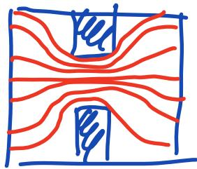
If we plot equally spaced contours of  $\psi$  the spacing indicates the speed of the flow.
