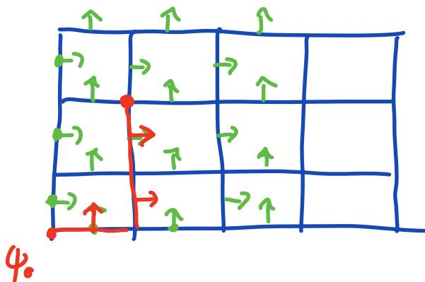
Given the location of  $v_x/v_y$  on the cell faces the natural location for  $\psi$  is on
