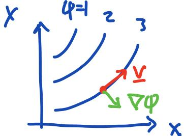
$$\begin{aligned}\nabla \psi \cdot \underline{v} &= \left( \frac{\partial \psi}{\partial x}, \frac{\partial \psi}{\partial y} \right) \cdot \begin{pmatrix} v_x \\ v_y \end{pmatrix} \\ &= (-v_y, v_x) \cdot \begin{pmatrix} v_x \\ v_y \end{pmatrix} = \\ &= -v_y v_x + v_y v_x = 0 \quad \checkmark\end{aligned}$$
