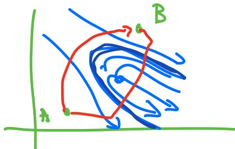
In an incompressible flow with out sources/sinks the cumulative flux  $\psi$  is a unique function of  $x$  and called the stream function.
