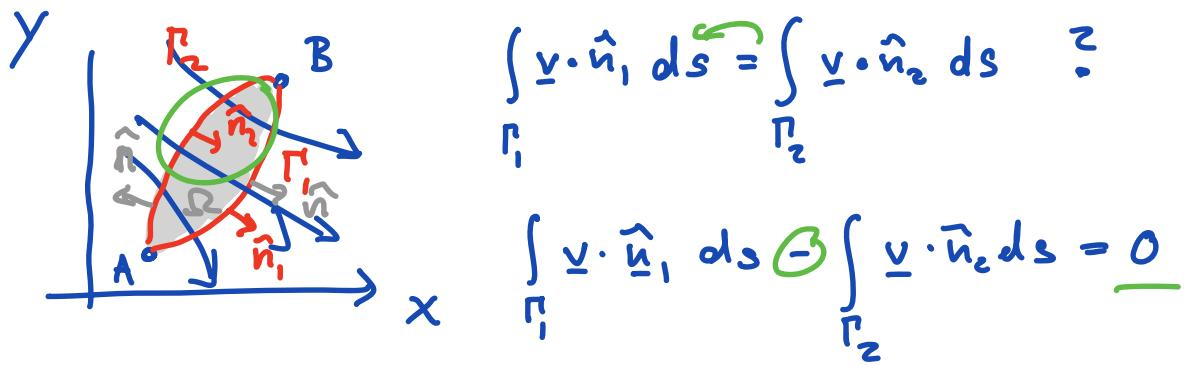
Combine  $\Gamma_1 + \Gamma_2 = \Gamma$  and define outside normal  $\hat{n}$  to the enclosed area  $\Omega$
