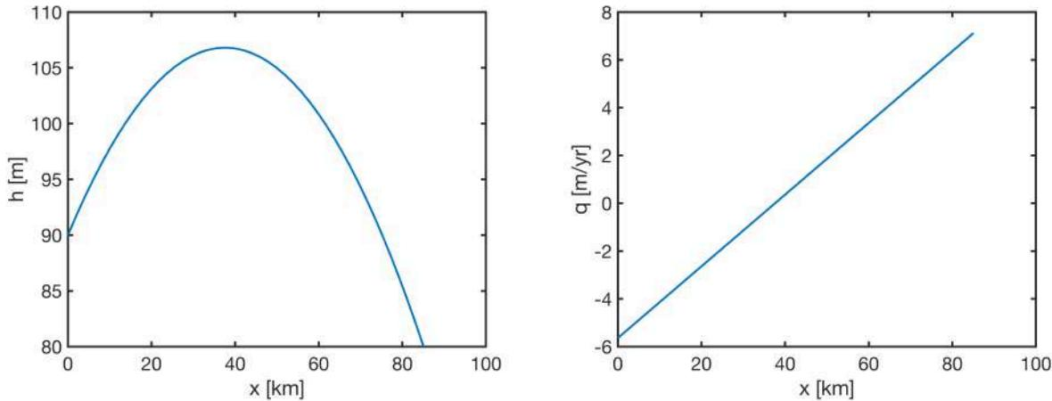
Previously we have imposed the heads of the two rivers as boundary conditions. Here we will evaluate the fluxes from the analytic solution at the boundary and then use them to prescribe the flux across the boundary rather than the head. This does not constrain the head on the boundary so we **must solve for the head on the flux boundary** and requires a different implementation of the boundary condition.
