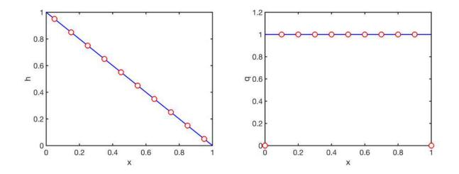
The flux computation fails on the boundary, because the gradient is set to zero by G.
