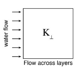
Now let's develop an analogous expression the effective hydraulic conductivity,  $K_{\perp}$ , for flow across the layers. In this case, the flux across each layer must be identical,  $q = q_n = -K_n \Delta h_n / l_n$ , but the head gradient across each layer  $\Delta h_n / l_n$ , will be different. The total head drop and the total medium length are then given by
