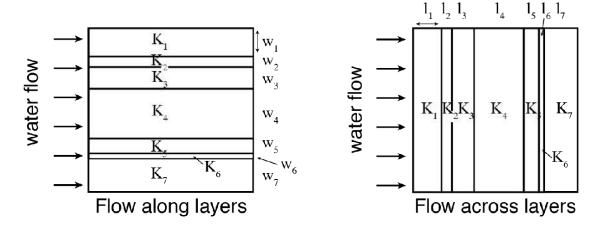
Consider a material with N layers, where the n-th layer has hydraulic conductivity,  $K_n$ , and width or length,  $w_n$  or  $l_n$ , depending on flow direction. The total width or length of the material are therefore
