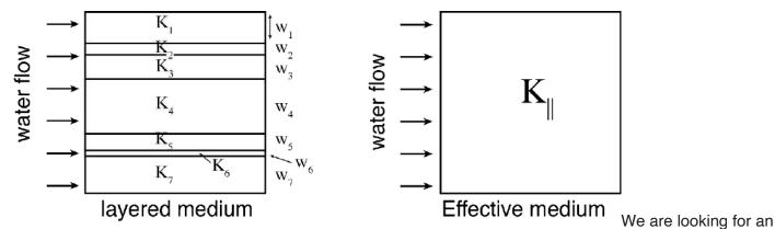
effective thermal conductivity,  $\kappa_{\parallel}$ , so that the total flow through the medium,  $Q=Wq=-W\,K_{\parallel}\frac{\Delta h}{L}$ , is identical
