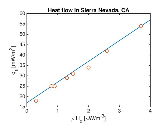
Here the slope of the data give  $h_r = 10 \text{ km}$  and the intercept  $q_m = 17 \text{ mW/m}^2$ . This suggests that between 5.5% and 68.5% of the surface heat flow is due to radiogenic heat production in the crust.
