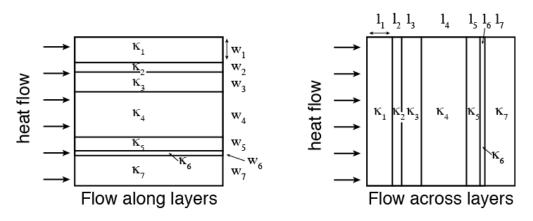
Consider a material with *N*layers, where the n-th layer has thermal conductivity,  $\kappa_n$ , and width or length,  $w_n$  or  $l_n$ , depending on flow direction. The total width or length of the material are therefore
